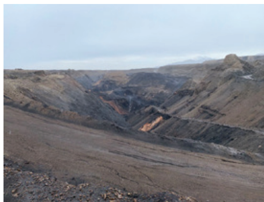
Outdoor Coal Mine under Spontaneous Combustion
